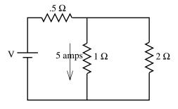
voltage divided by 2  $\Omega$ 's, or i = (5 volts)/(2  $\Omega$ ) = 2.5 amps, and the total current into the parallel combination (i.e., the current through the .5  $\Omega$  resistor) is 2.5 amps + 5 amps = 7.5 amps. With that, we can write: V<sub>.5 $\Omega$  res</sub> = (7.5 amps)(.5  $\Omega$ ) = 3.75 volts. This response is false.]
